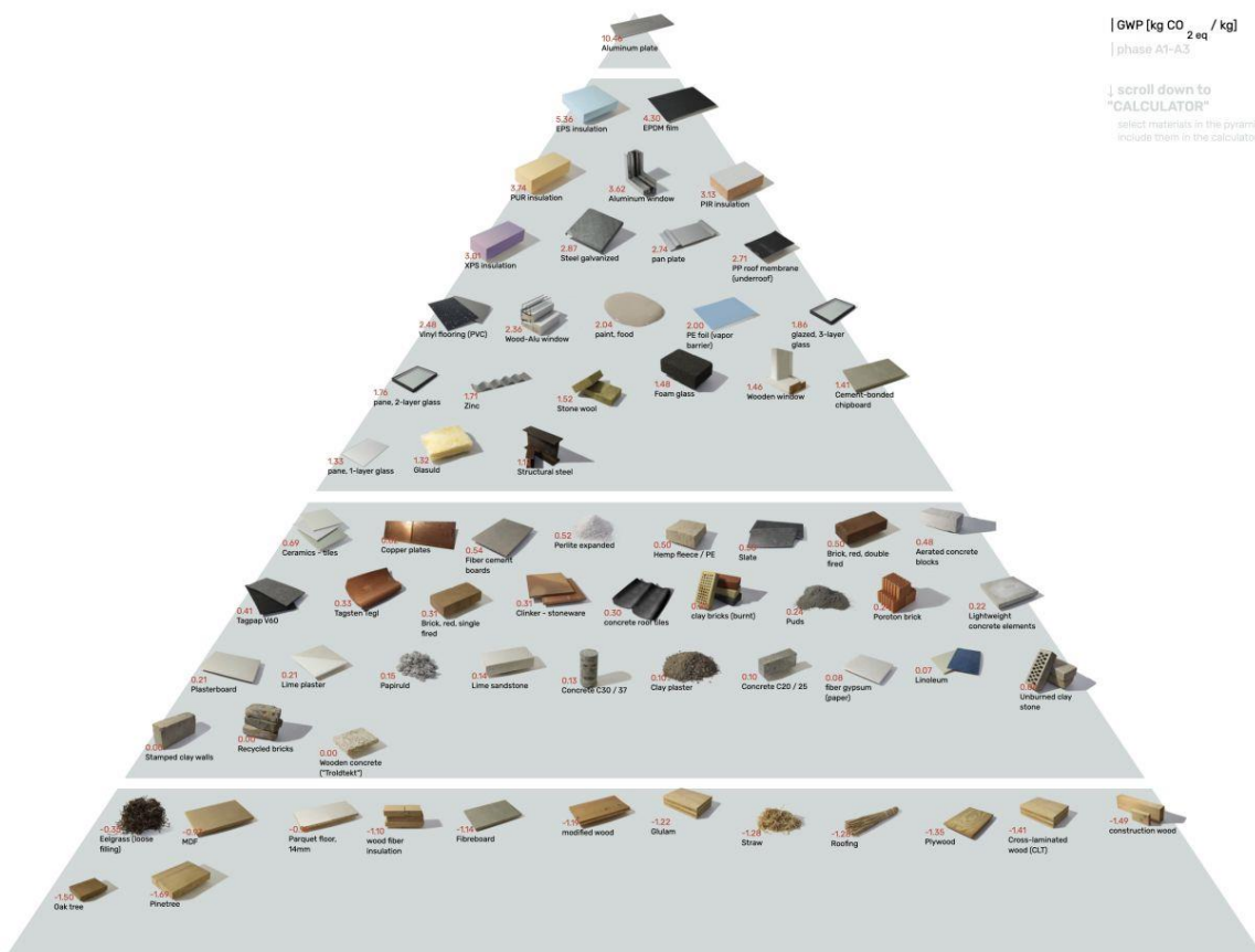
Milieu Impact van bouwmaterialen. Bron: Cinark (2020). Center for Industrialised Architecture Royal Danish Academy
